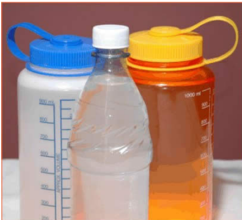
When selecting plastic water bottles, #2 HDPE (left), #4 LDPE & #5 PP bottles are good choices. #1 PET/PETE bottles (center) are not recommended for repeat use due to the risk of bacterial contamination. Clear, hard #7 polycarbonate bottles (right) may leach an artificial estrogen.
